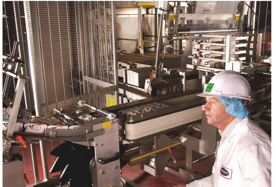
Cartons of ice lollies, or ice cream novelties for various Nestlé brands, left and right, above, are handled on a new type of shrink wrapper that relies less on tension and heat energy and more on the efficiency and improved design of the shrink tunnel.
