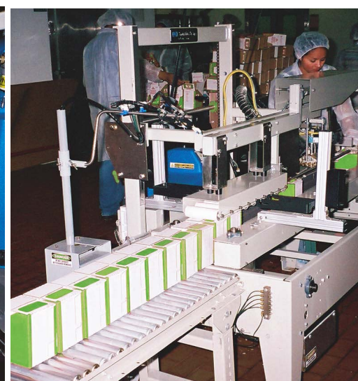
Carton erector, left, picks knocked-down cartons from the feed magazine, erects them and seals the bottom flaps with hot-melt glue. Top sealer, above, closes top flaps and seals them with hot-melt glue.
