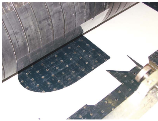
Here, the film window (on the roller) is scored and affixed to the finished carton blank by a special window-application machine.
